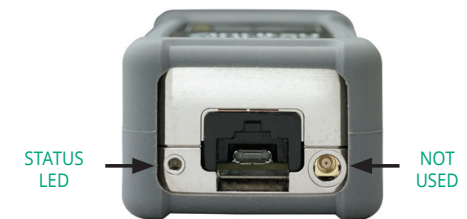
MICRO USB CONNECTOR WITH LATCH
